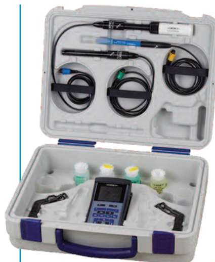
Set in a Field Case with Multi 3430 IDS meter and IDS pH, Cond, and DO sensors
